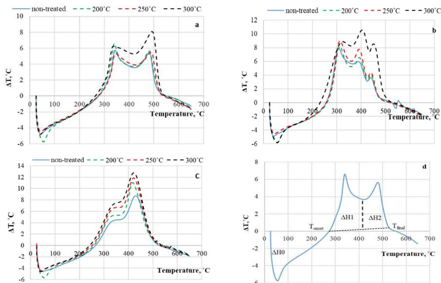
Fig. 2. DTA profiles in air for non-treated and MW torrefied biomass of different origin: softwood (a), wheat straw (b) and peat (c); principle of heat effect calculation using DTA exemplified by non-treated softwood ( $\Delta H$  – normalized area;  $T_{onset}$  and  $T_{final}$  – first and last point of integration range, respectively)
