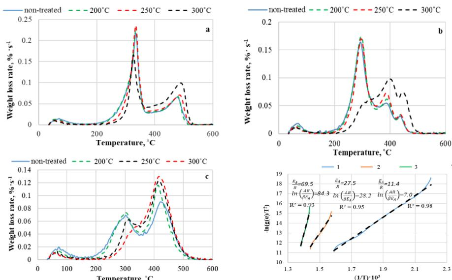
Fig. 1. DTG profiles in air for non-treated and MW torrefied biomass of different origin: softwood (a), wheat straw (b) and peat (c); linear regression in Coats-Redfern coordinate for different degradation zones of non-treated wheat straw (1 – volatilization stage; 2, 3 – char combustion stage) (d)
